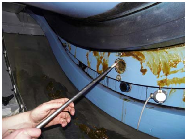
Figure 17: A Type II Grease Thief is prepared on a T-handle extension to obtain a main bearing sample from the purge drain. (Oelcheck Labs, Germany)
