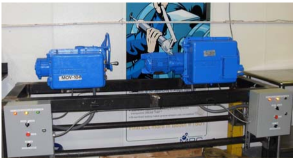
Figure 5: Motor Operated Valve (gearbox) test stand
