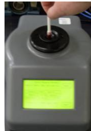
Figure 8: Hall-effect (FdM+) sensor and Grease Thief
