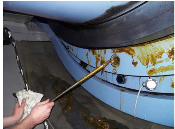
Figure 18: The full Grease Thief is removed from the drain of a 2MW wind turbine, and can be submitted for streamlined routine analysis for grease and bearing condition assessment. (Oelcheck Labs, Germany)
